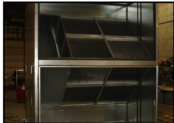
Exchanger, with bypass air channel on the left
