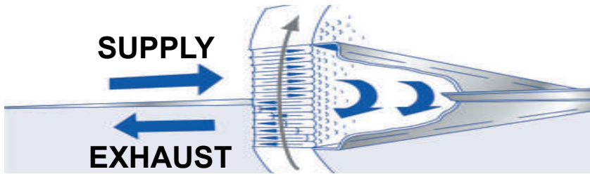
Xetex Series-S Purge Sector. The angle of the purge sector is custom designed according to the specific conditions of each application.
