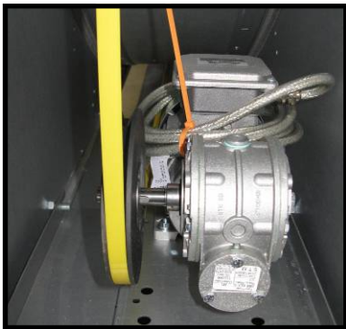
A 1/3 to 1 hp gear reduced motor with soft-start requires no maintenance as all components are pre-lubricated and sealed.
