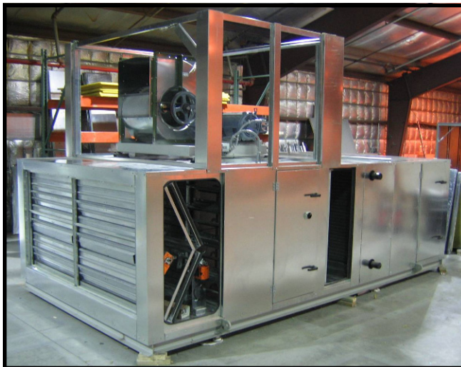
Top level blower cabinet is configured for exhaust air out. Supply air enters the bottom section through the damper (left) and flows out the other end (right).
