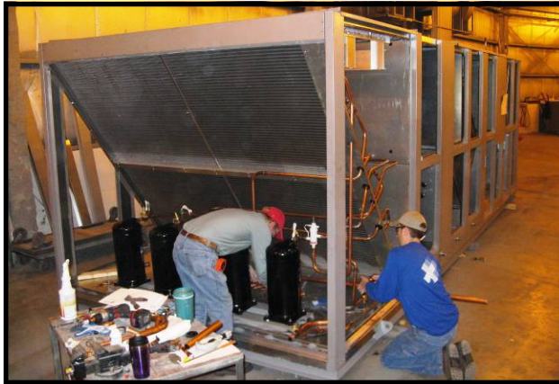
The entire DX circuit is plumbed and wired by XeteX.
