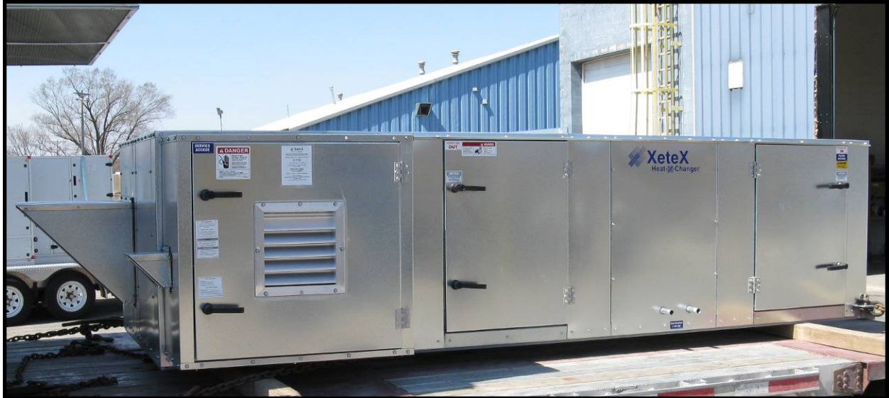
A fully-assembled IAQ-B. This unit has an integral indirect gas-fired heater and is configured for roof top installation with 1" thick double-wall construction and an all-welded galvanized steel drain pan.
