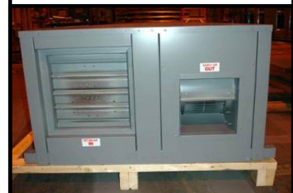
End views of an IAQ-500D. Exhaust air (top left) and supply air (bottom right) blower outlets are visible along with outdoor air (top right) and return air (bottom left) backdraft damper inlets.
