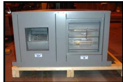
End views of an IAQ-500D. Exhaust air (top left) and supply air (bottom right) blower outlets are visible along with outdoor air (top right) and return air (bottom left) backdraft damper inlets.
